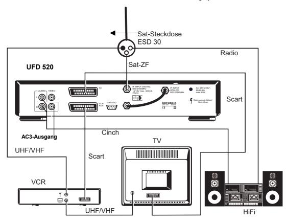
Connection of the DVB-S receiver to a TV set, a VCR and a hi-fi system for receiving and recording digital satellite TV and radio channels. The digital sound output can be connected to a Dolby Digital system.
